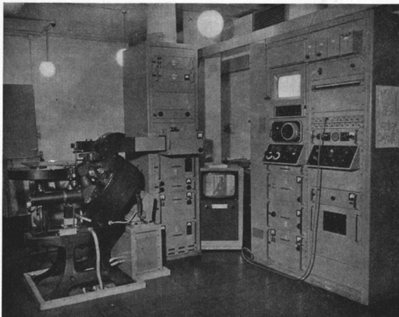
Fig. 14 — 35-mm. Flying Spot Mechau Telecine Equipment
