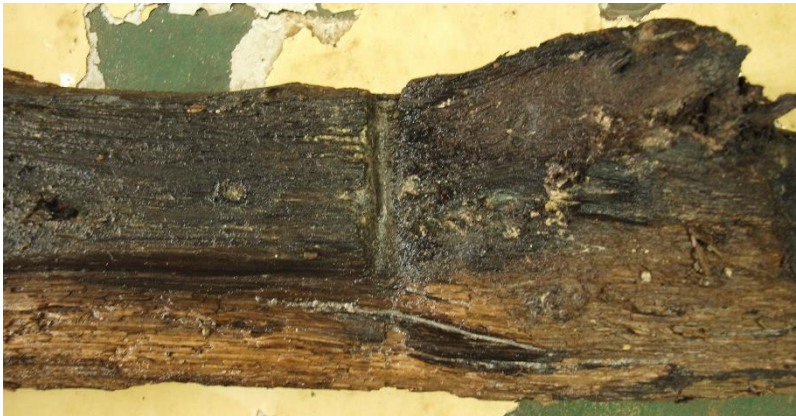
Plate 5 The dent made by the machine
