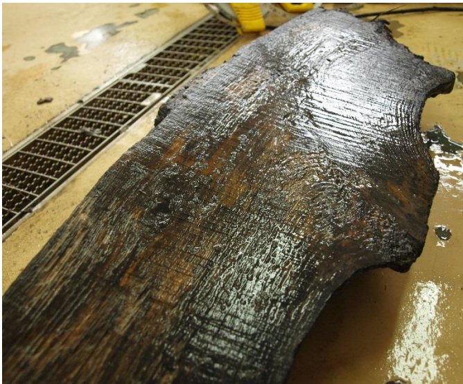
Plate 3 Saw marks on worked side of timber
