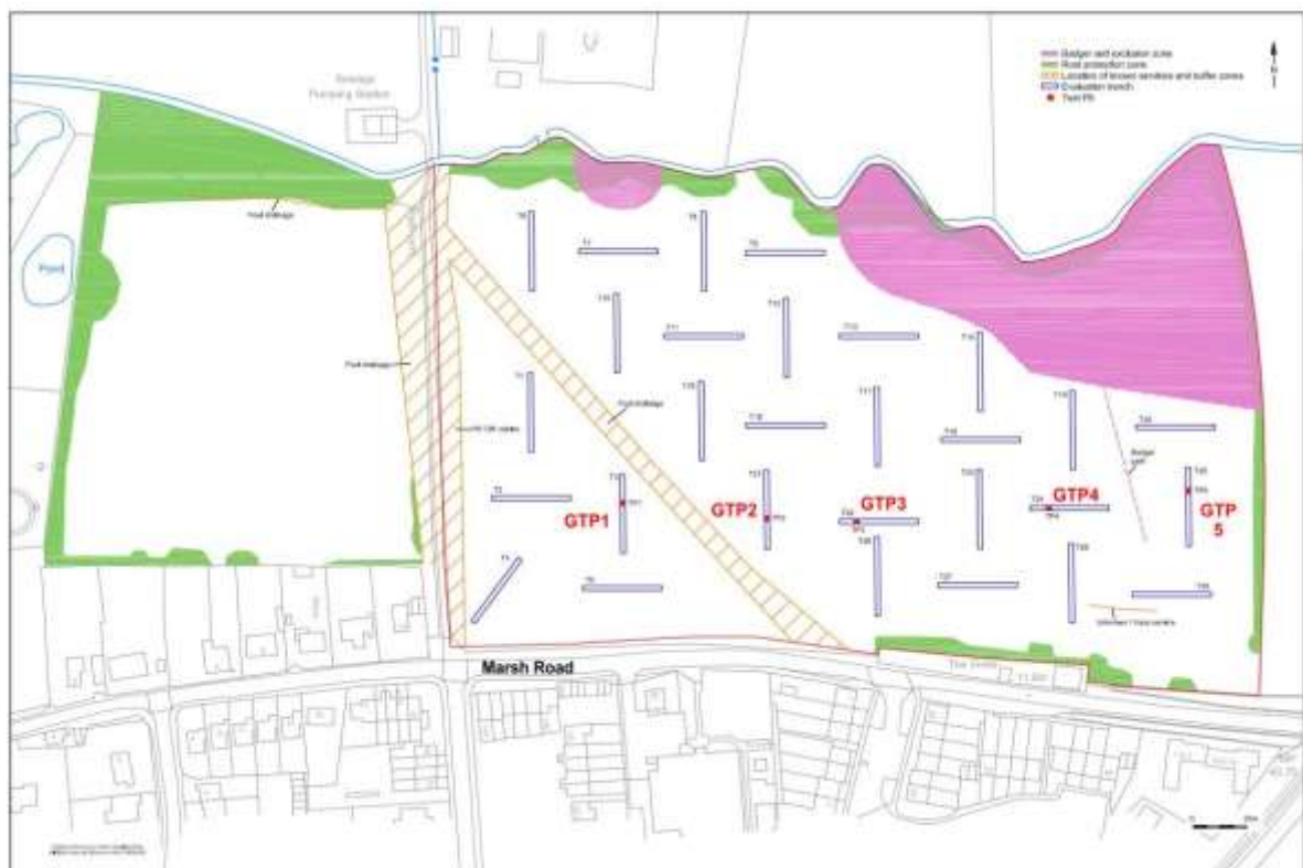
Figure 6: Locations of archaeological and geotechnical trial pits on site (reproduced from Archaeology South East)
