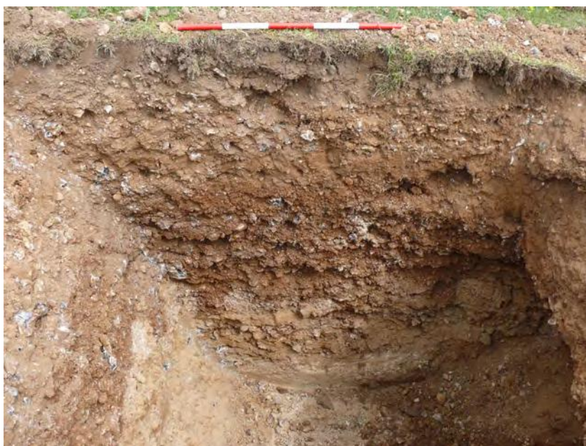
Fig. 13: GTP7 north facing section. Made ground, fluvial gravel and gelifluction deposits
