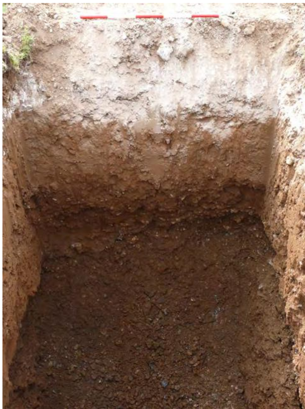
Fig. 12: GTP1 south-east facing section. Made ground, colluvium and fluviat gravel
