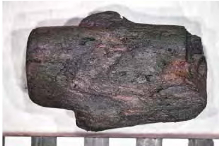
2: Internal surface along longitudinal split showing conical recess at right hand end
