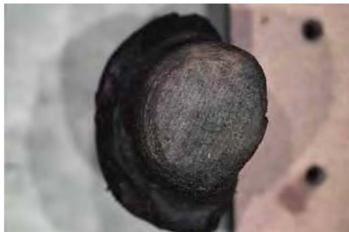
4: Sawn end showing parallel saw marks
