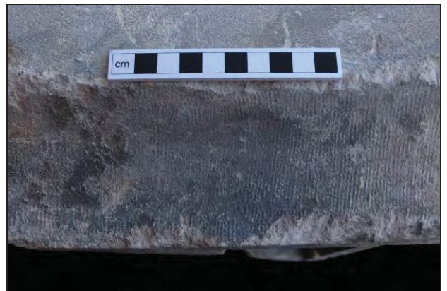
Detail of tooling marks
