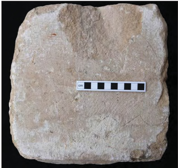
Edge with setting out lines for round moulding
