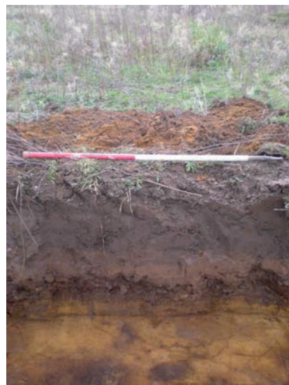
DP 4: Sample section showing podsol and iron hard pan layers
