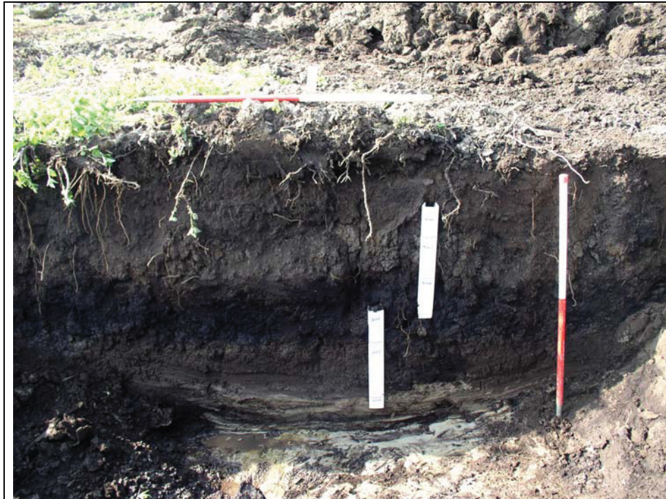
Plate 3: Location of column sample taken from Test Pit 1, showing sequence (upwards from base) of natural Kimmeridge Clay, alluvial silt, lower peat, upper peat, subsoil and topsoil.
