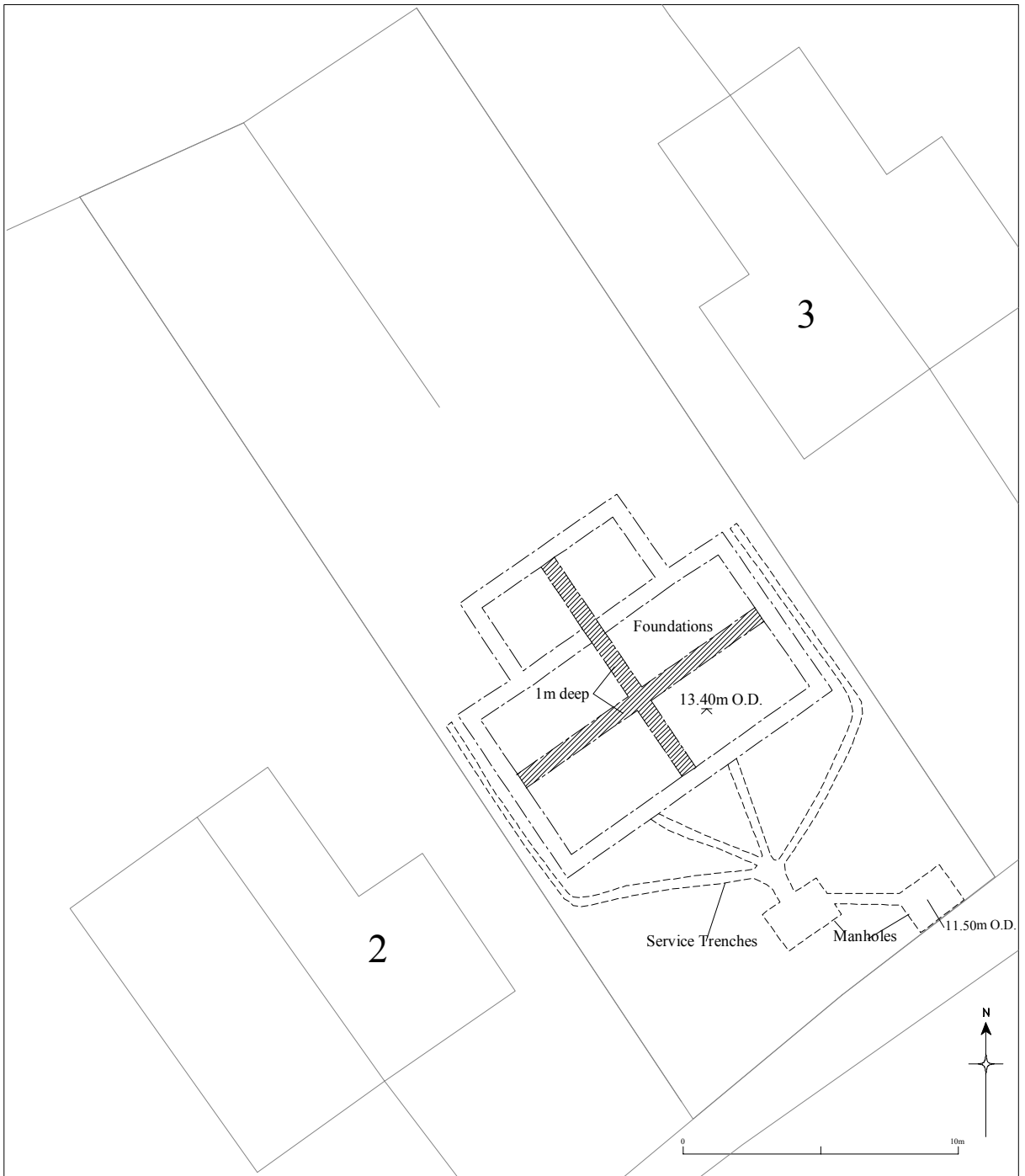
Figure 2 Plan showing the position of the excavated foundations and service trenches within the development
