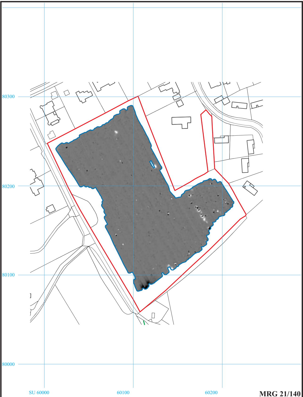
Land east of Manor Road, Goring-on-Thames, Oxfordshire, 2021 Geophysical Survey (Magnetic) Figure 2. Plot of raw gradiometer data.
