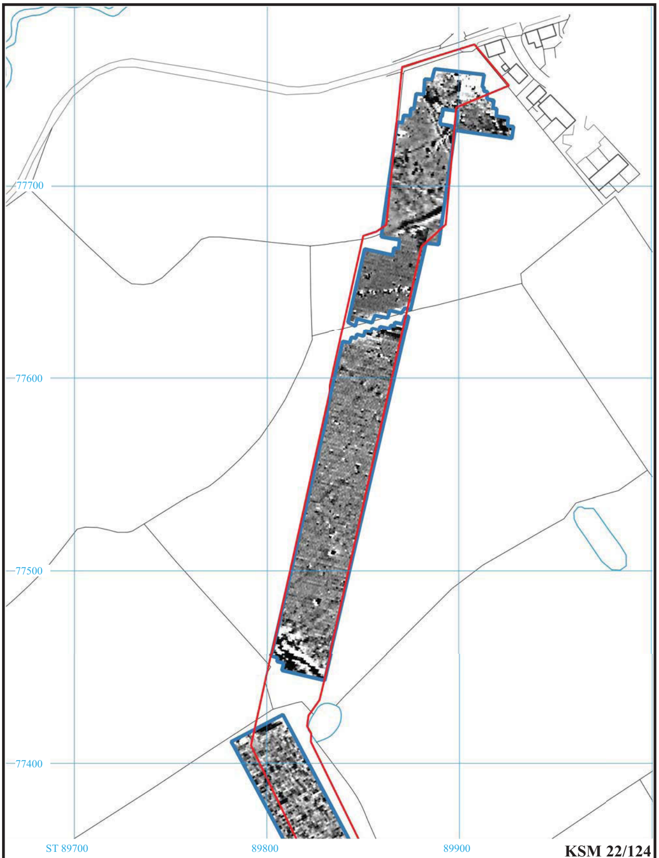
Mains Replacement Pipeline, Kington St. Michael Wiltshire, 2022 Geophysical Survey (Magnetic) Figure 8. Focused plot of processed gradiometer data (north).
