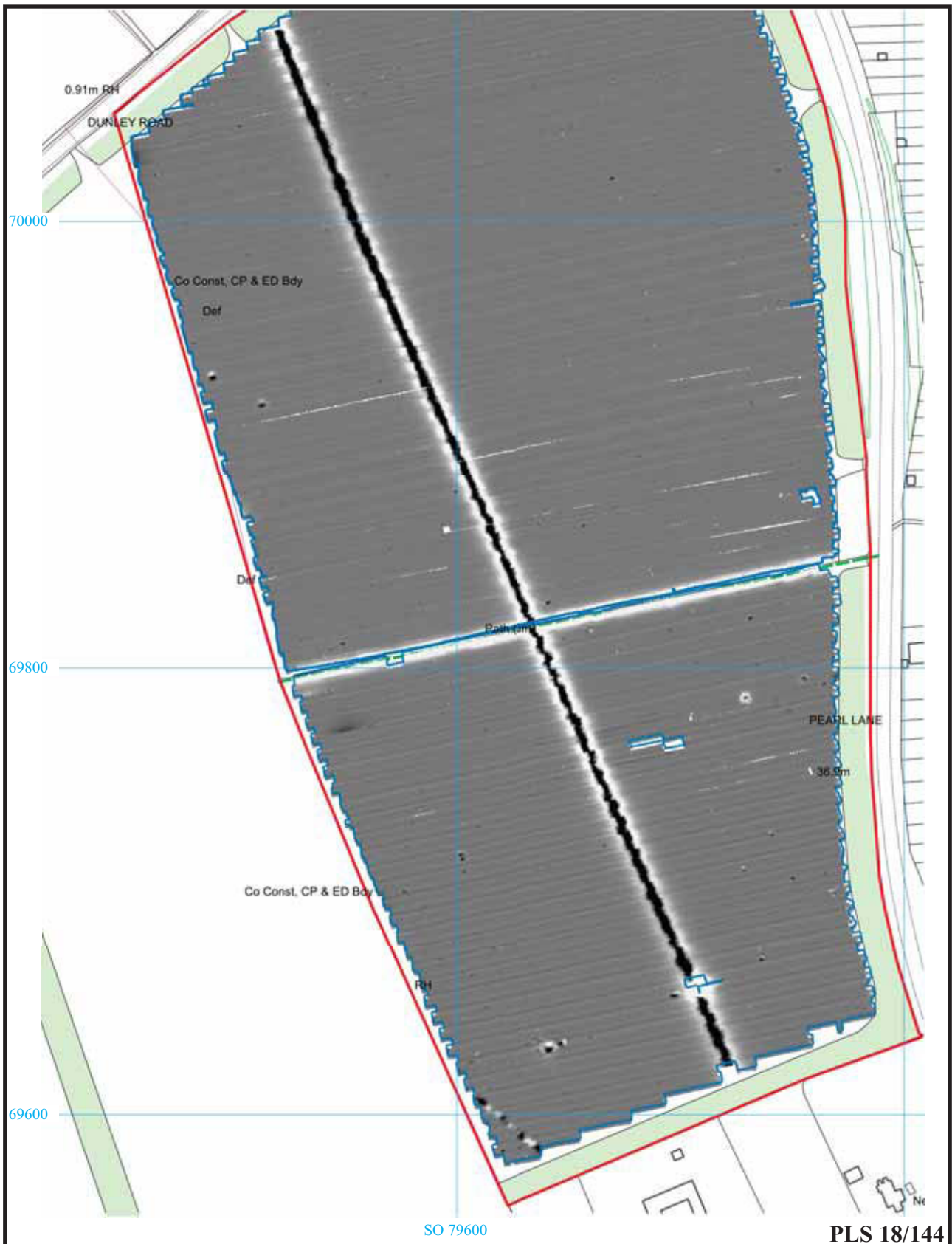
Land at New Barns Farm, Pearl Lane, Stourport, Worcestershire, 2018 Geophysical Survey (Magnetic) Figure 4. Plot of raw gradiometer data (south).
