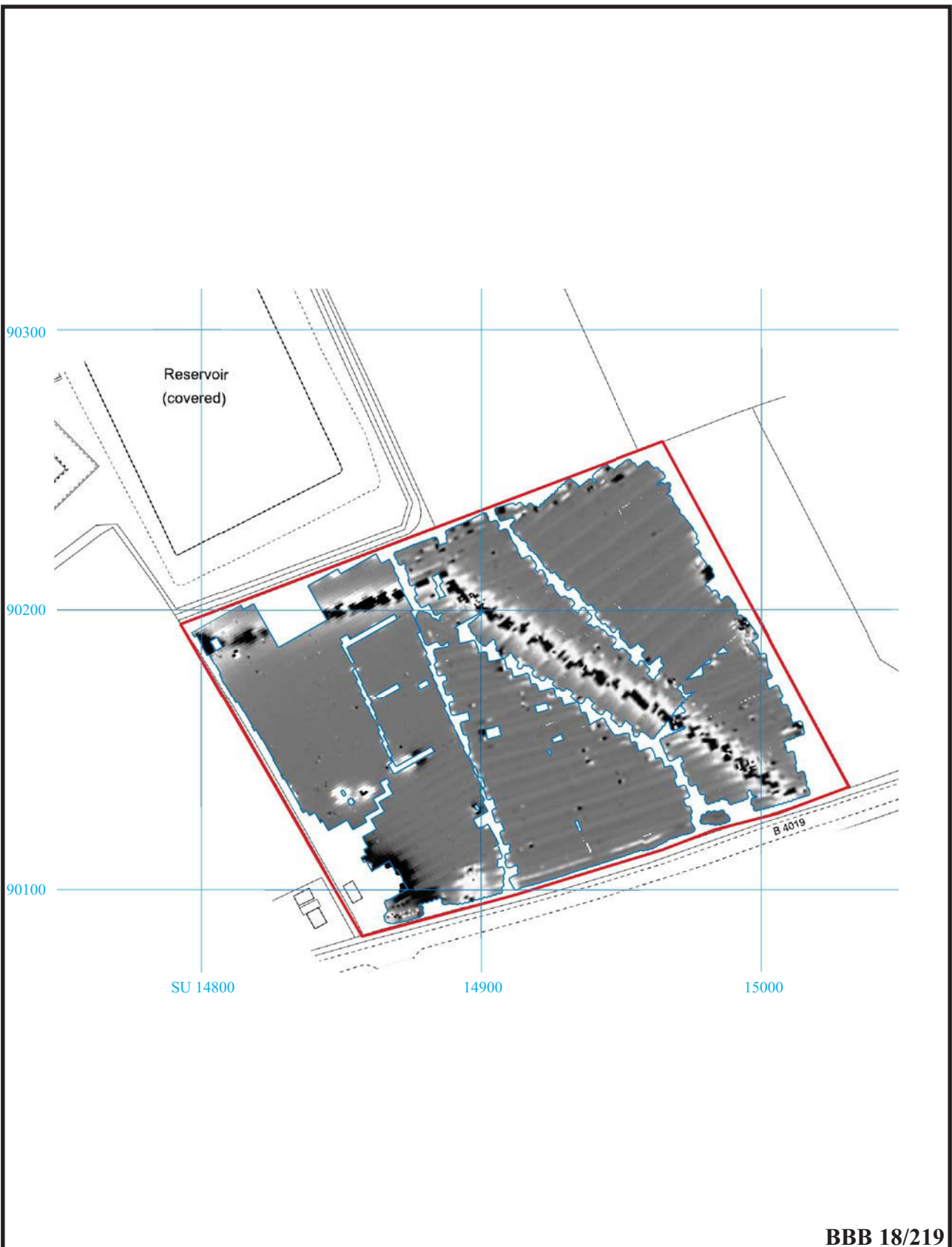
Land off B4019, Broad Blunsdon, Swindon, Wiltshire, 2019 Geophysical Survey (Magnetic) Figure 2. Plot of raw gradiometer data.
