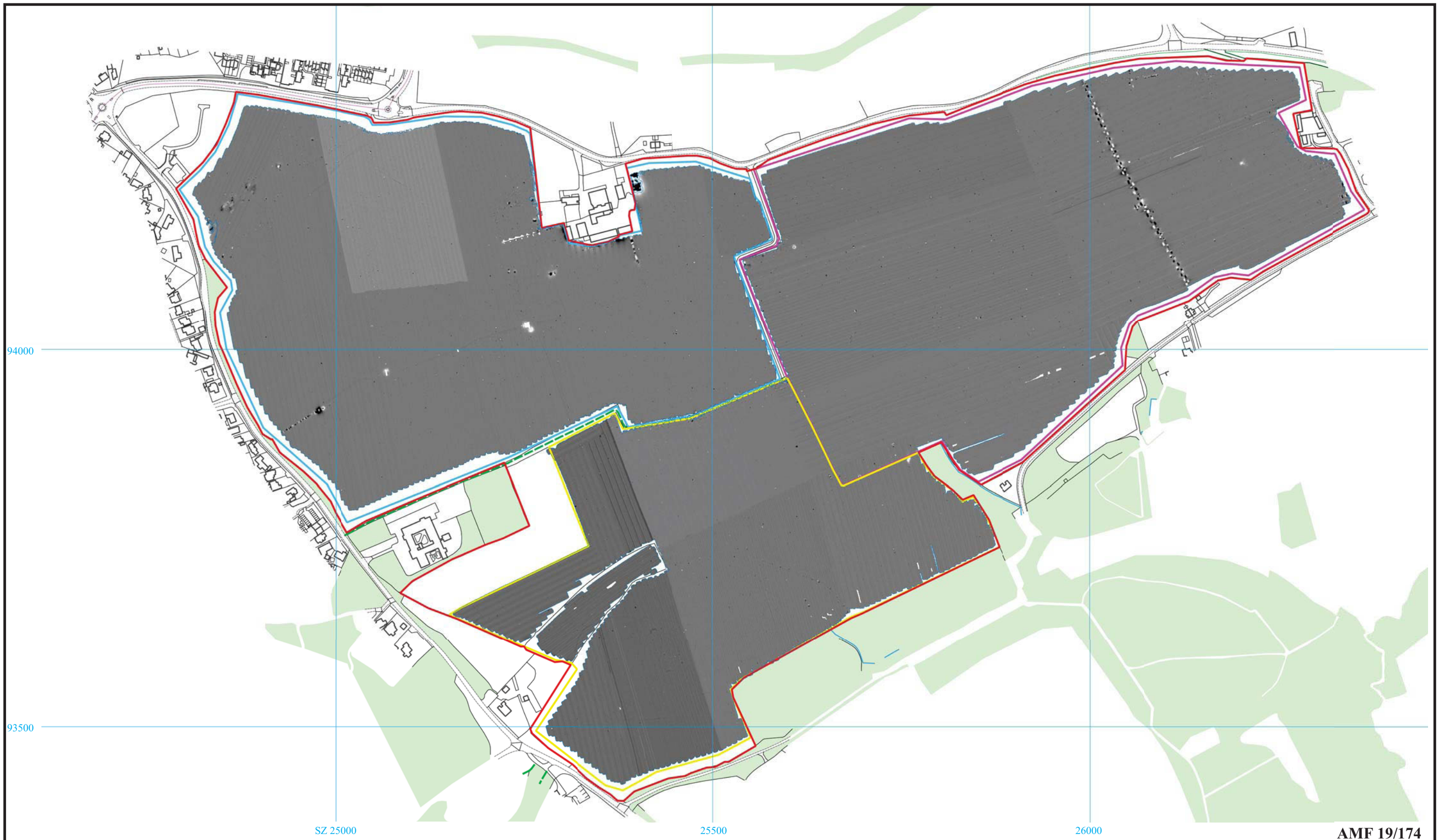
Ashley Manor Farm, Lymington Road, New Milton, Hampshire, 2019 Geophysical Survey (Magnetic) Figure 2. Plot of raw gradiometer data.
