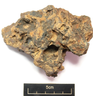
Figure 3. Furnace slag (with abundant charcoal impressions [809] (893)
