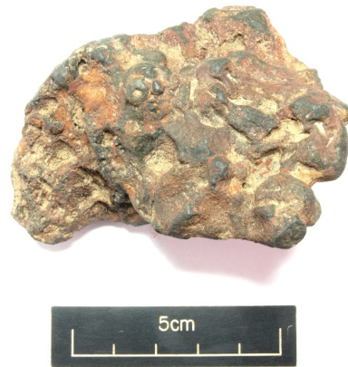
Figure 4. Eroded furnace slag (with abundant charcoal impressions [316] (458)
