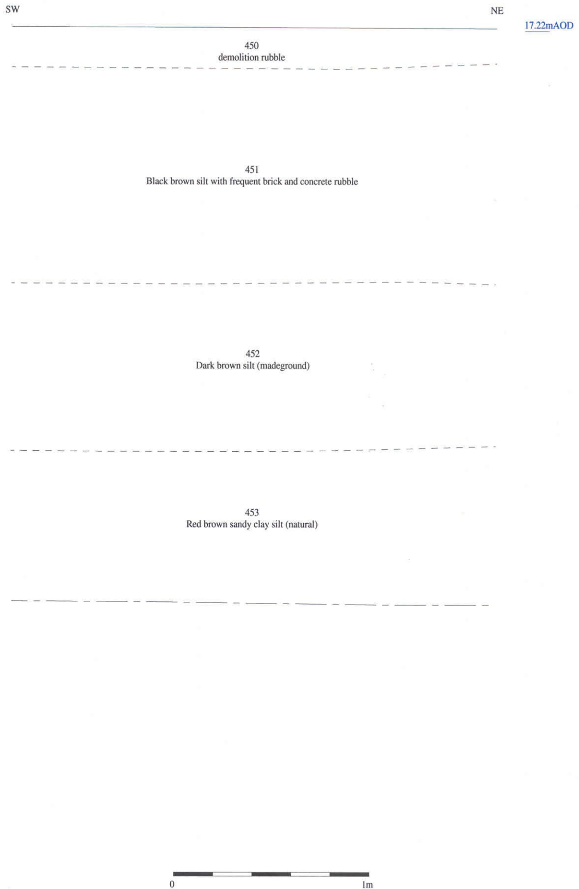
Figure 4. Representative section of borrow pit excavation.
