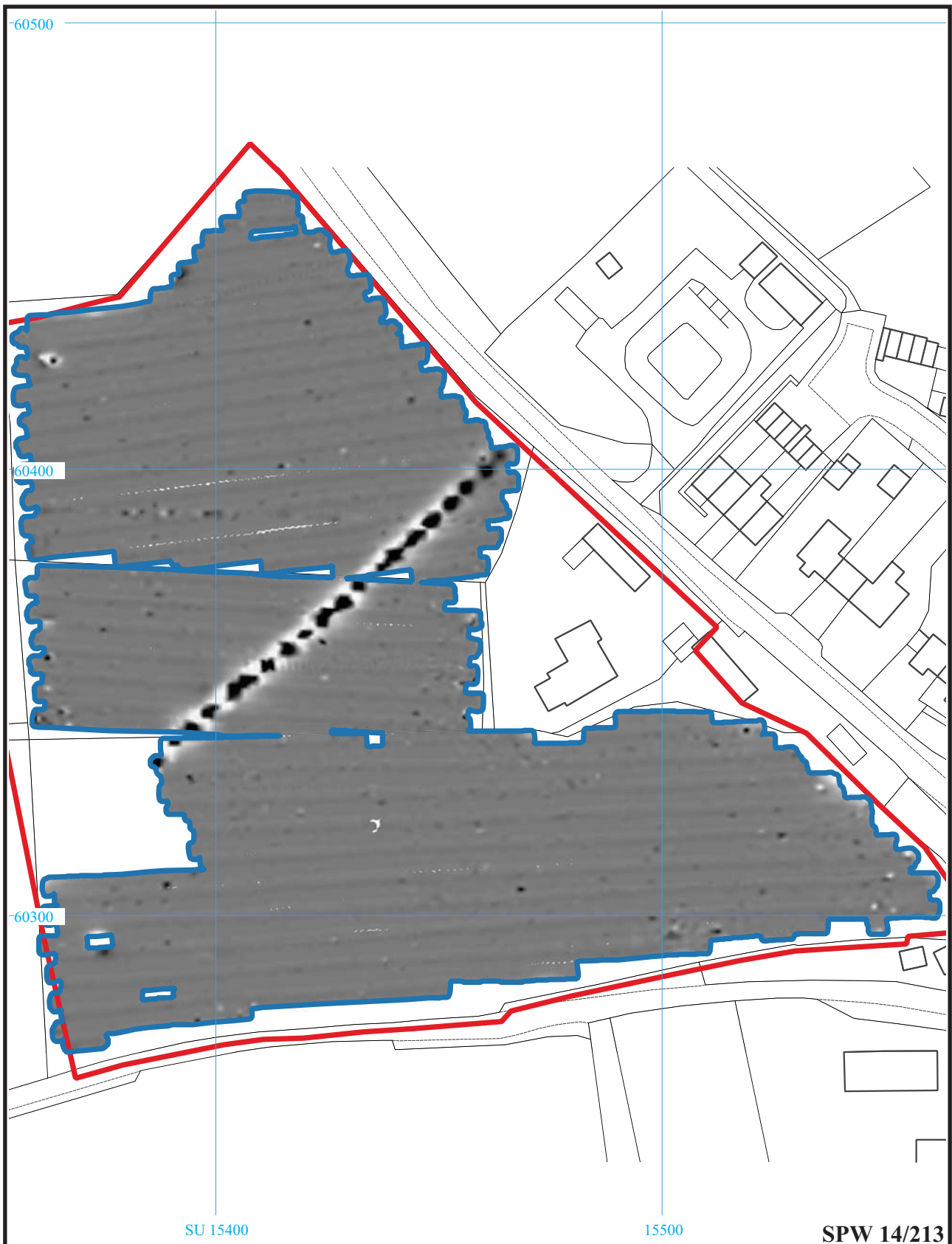
Land off Wilcot Road, Stonington, Pewsey, Wiltshire, 2020 Geophysical Survey (Magnetic) Figure 2. Plot of raw gradiometer data.
