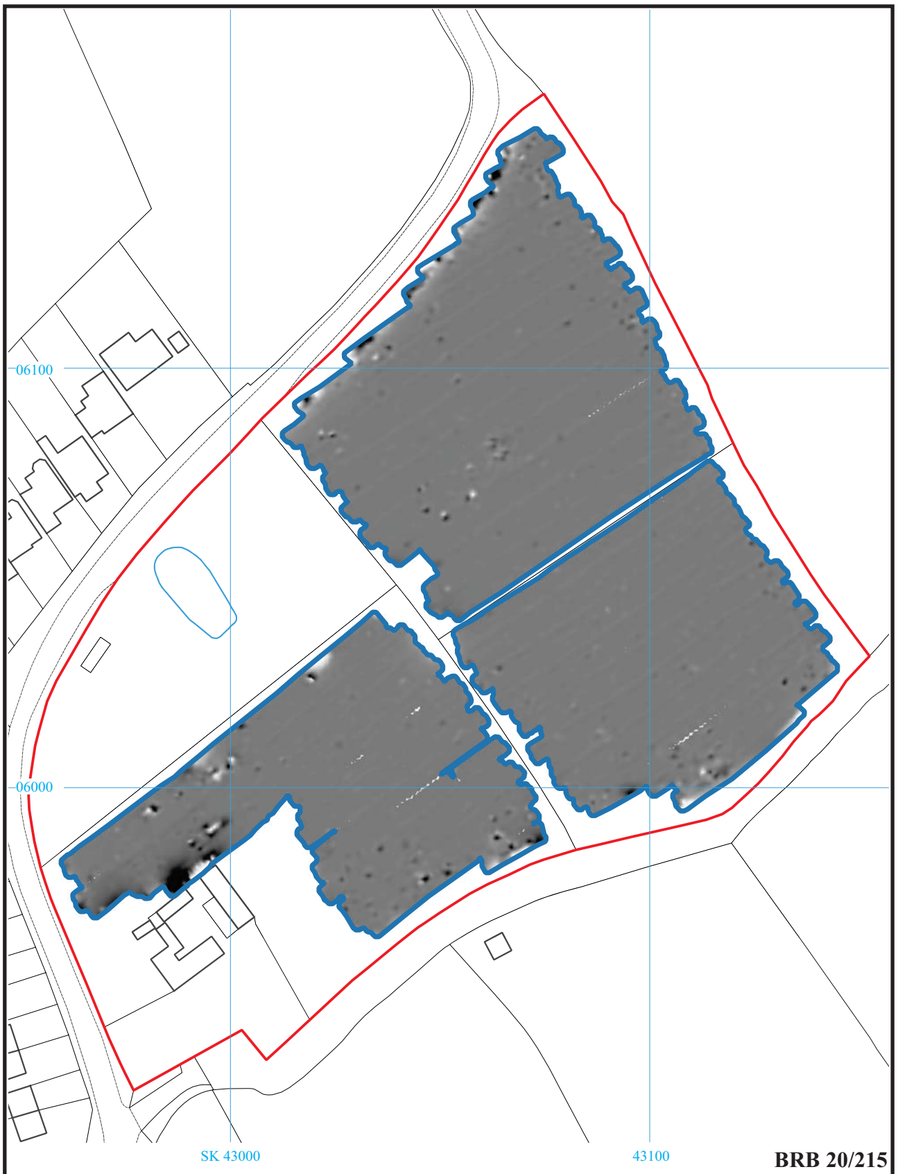
Land off Bagworth Road, Barlestone Leicestershire, 2021 Geophysical Survey (Magnetic) Figure 2. Plot of raw gradiometer data.
