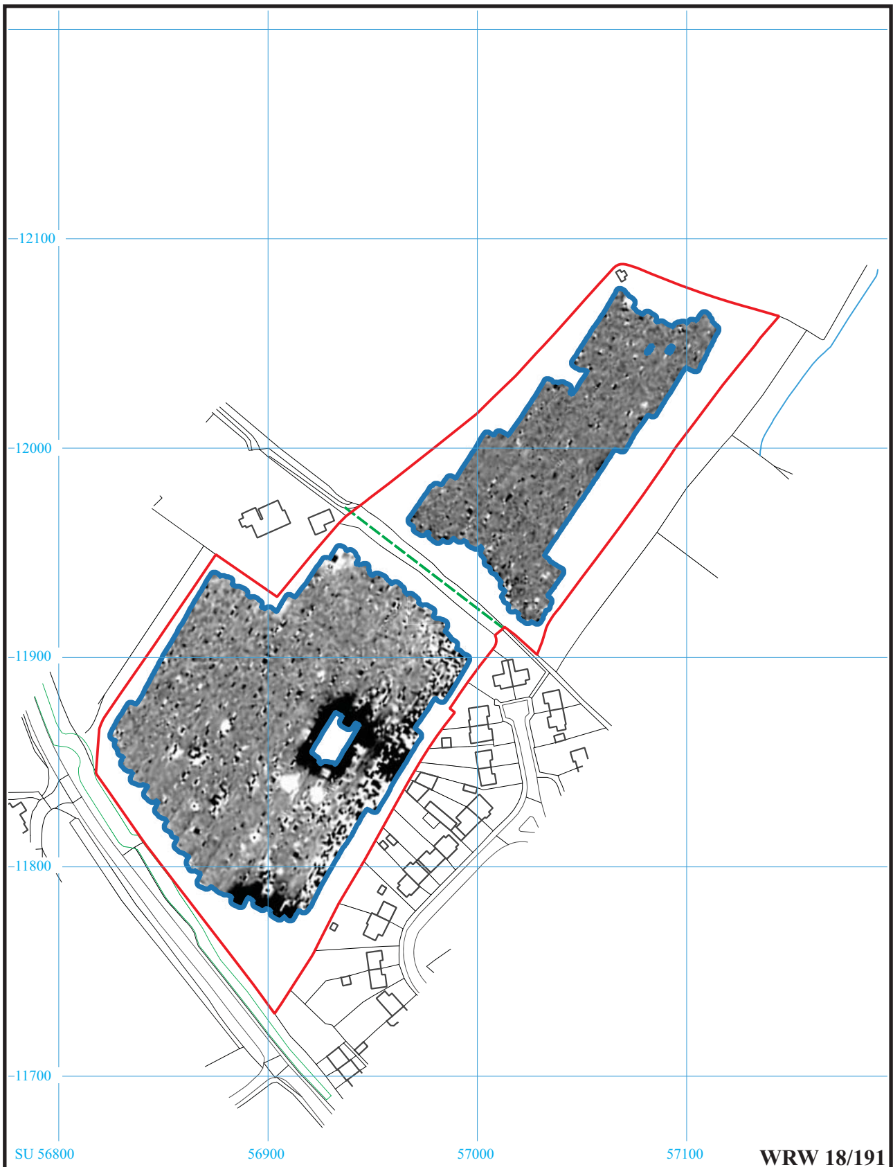
Land at Winchester Road, Wickham, Hampshire, 2021 Geophysical Survey (Magnetic) Figure 3. Plot of processed gradiometer data.
