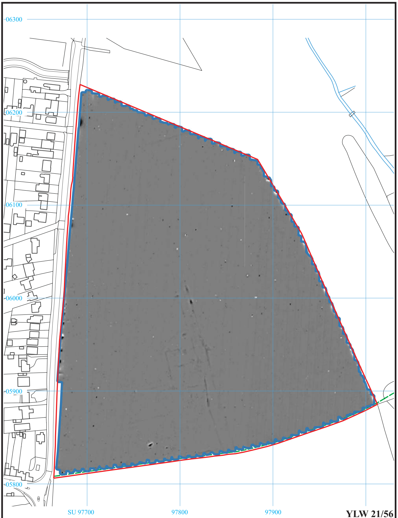
Land east of Yapton Lane, Walberton, West Sussex, 2021 Geophysical Survey (Magnetic) Figure 2. Plot of raw gradiometer data.
