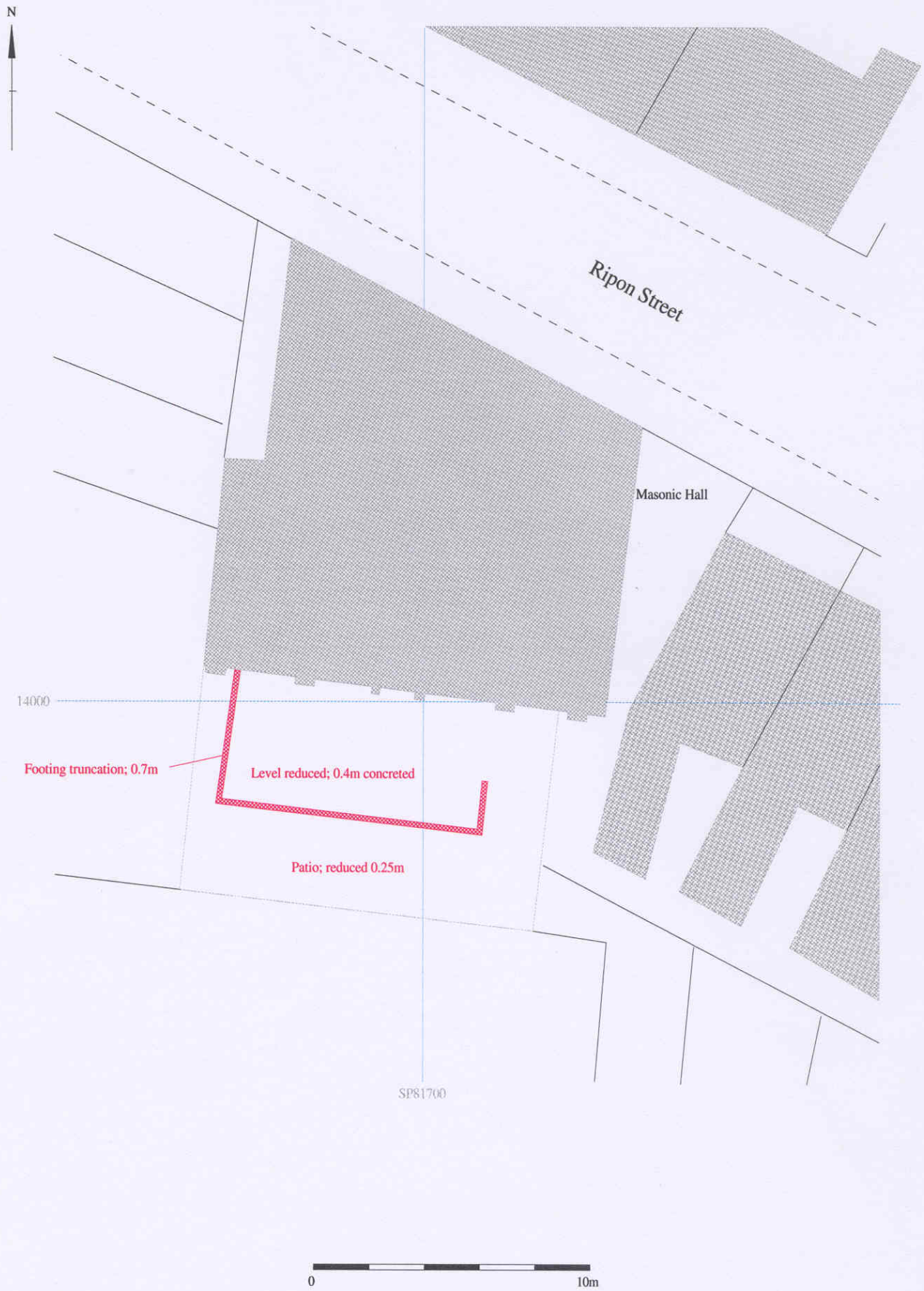
Figure 3. Areas affected by groundworks.
