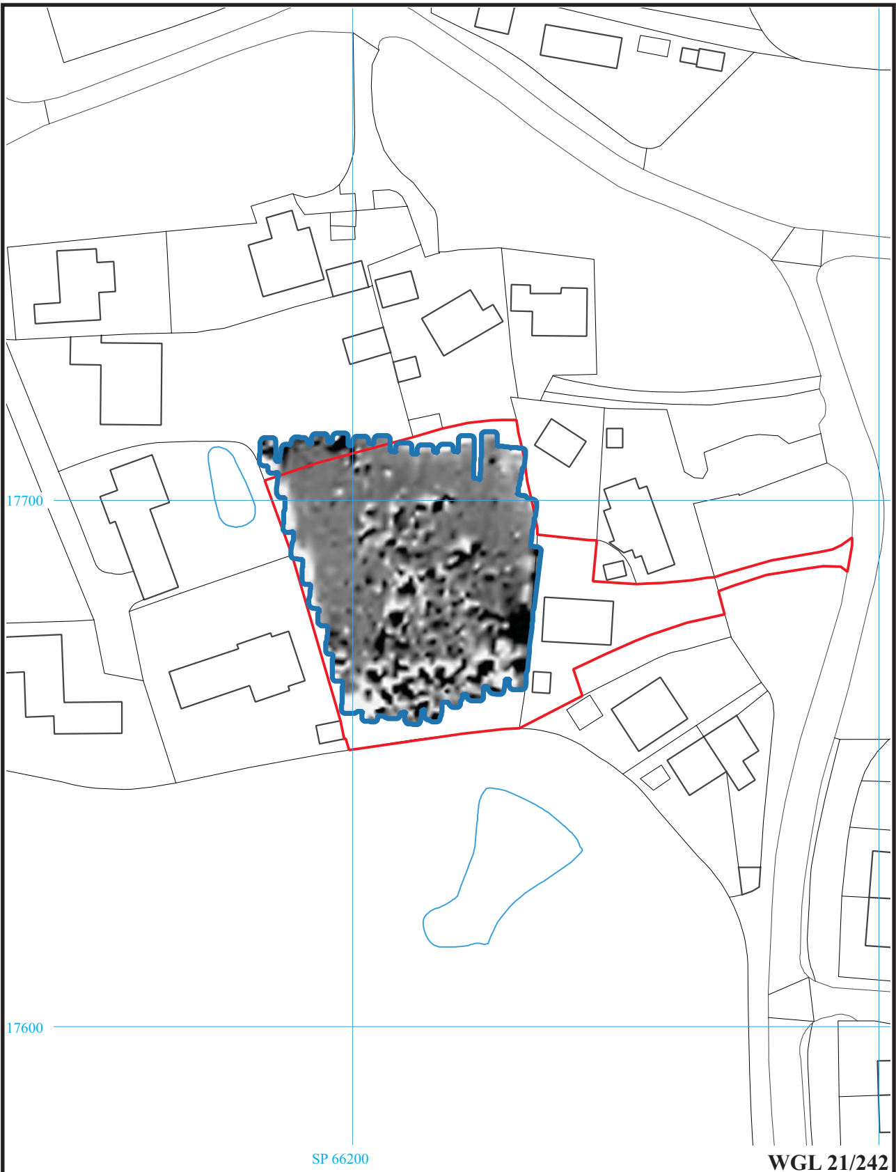
Land at Westhaven and Green View, The Green, Ludgershall, Buckinghamshire, 2021 Geophysical Survey (Magnetic) Figure 3. Plot of processed gradiometer data.
