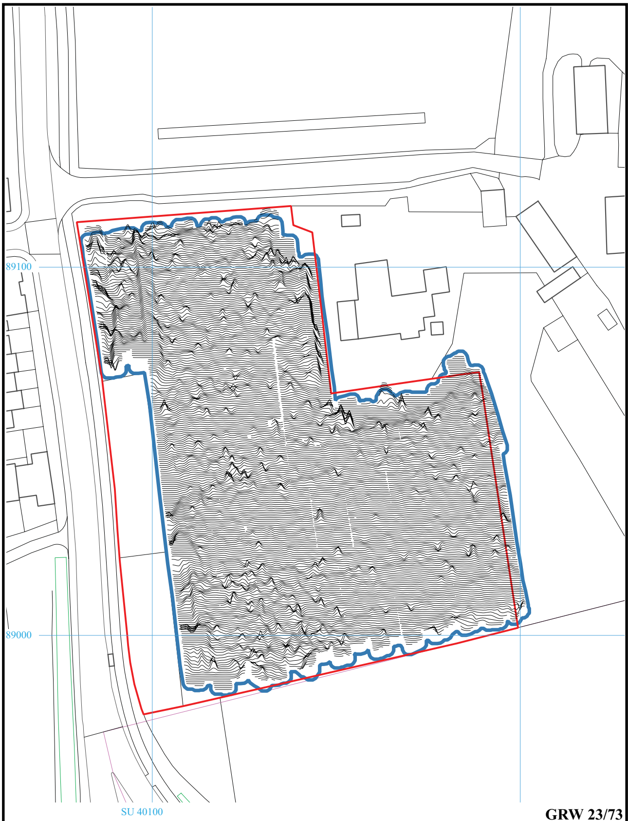
Land at Grove Road, Wantage, Oxfordshire, 2023 Geophysical Survey (Magnetic) Figure 5. XY Plot of processed gradiometer data.
