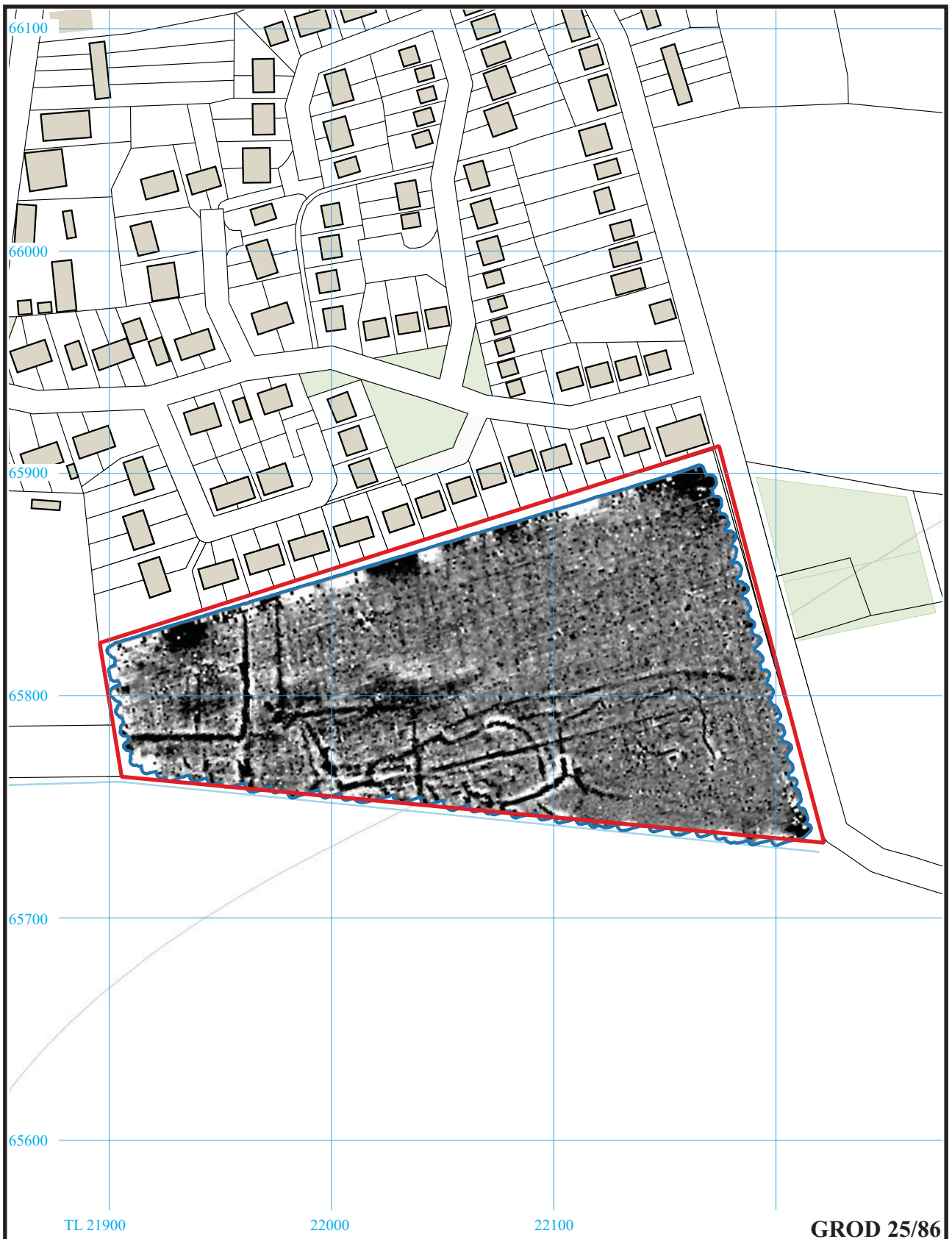
Land off Graveley Road, Offord D'Arcy, Cambridgeshire, 2025 Geophysical Survey (Magnetic) Figure 4. Plot of processed gradiometer data.
