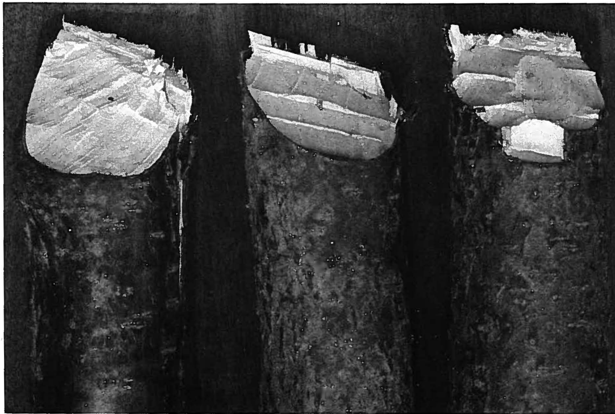
Fig. 16 Hazel rod chopped at medium angles with (left) a flat bronze axe, (centre) a palstave, and (right) a socketed axe. The flat axe left rather indistinct facets, and 51 blows were delivered on this face. The palstave left 3 clear facets from 57 chops. The socketed axe was light in weight and to produce this set of 7 facets took 207 chops. Diameter of the hazel rod 37–39mm, age 10 years. Scale \frac{1}{2} .
