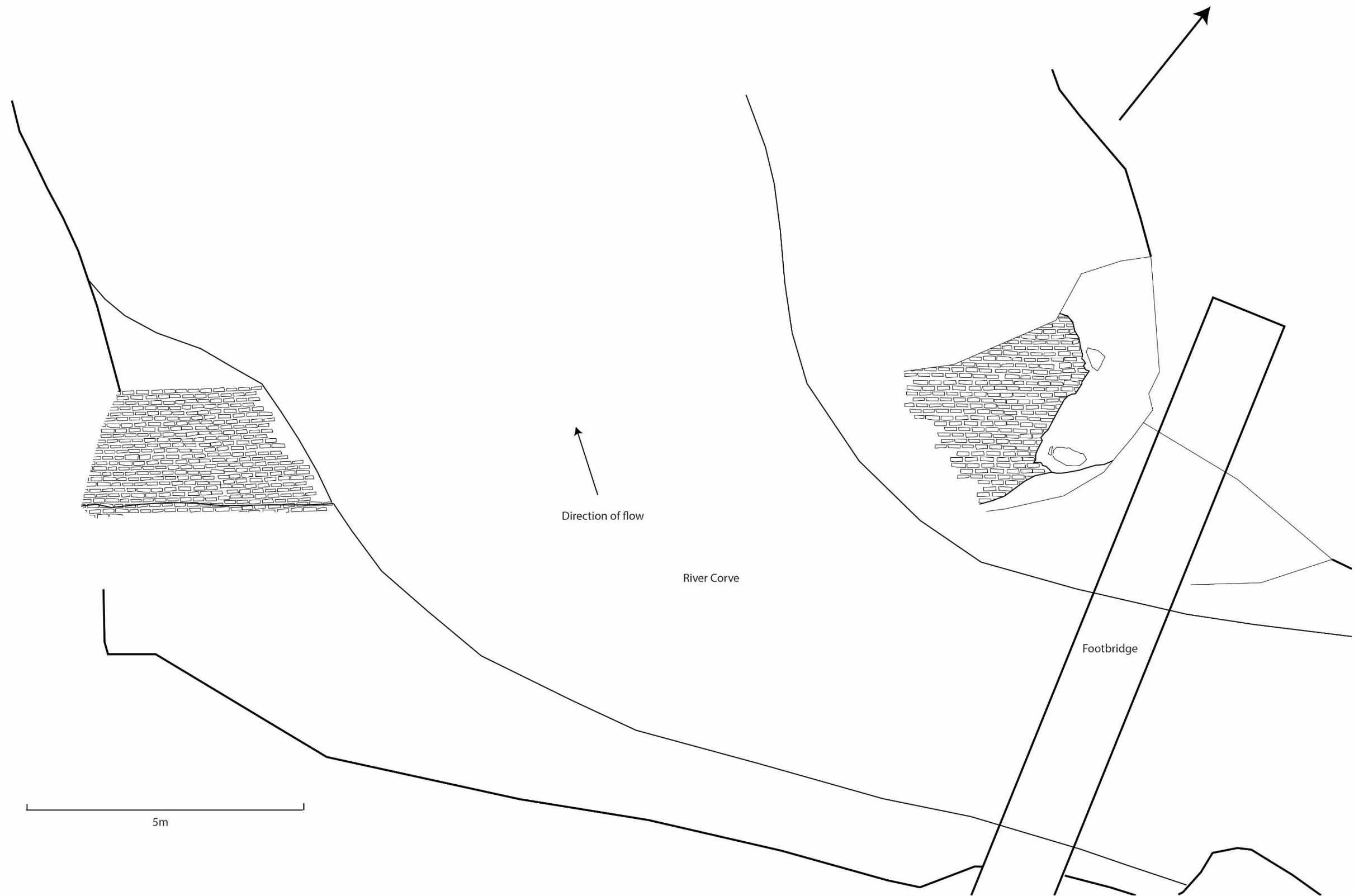
Fig. 16 Plan following removal of the central section of the weir
