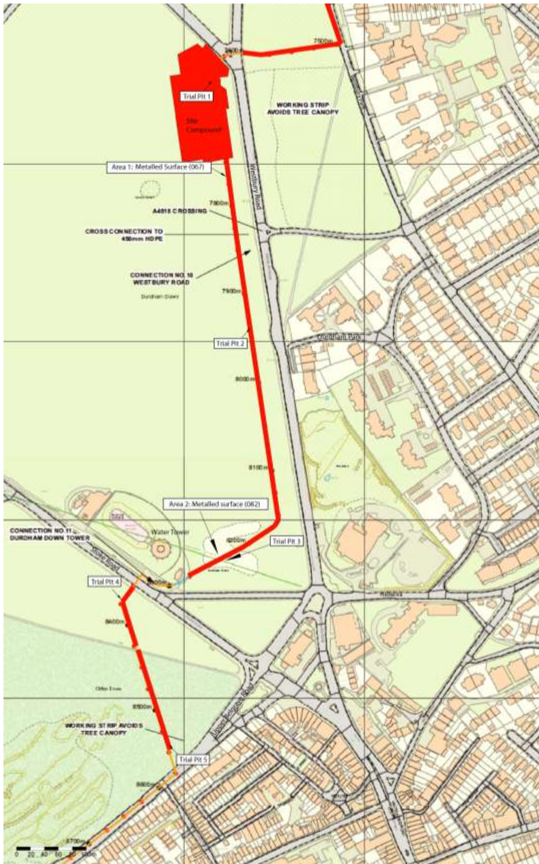
Fig. 3: Scheme plan showing easement route and location of areas of further investigation & recording in the NE corner of Durdham Down (Area 1) and to the E of the Water Tower on Stoke Road (Area 2)
