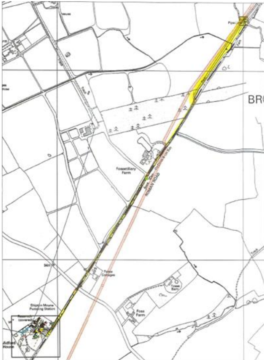
Fig 1: Plan showing the route of the pipeline from Shipton Moyne Pumping Station to the River Avon (marked in yellow) with an existing gas pipeline marked in red
