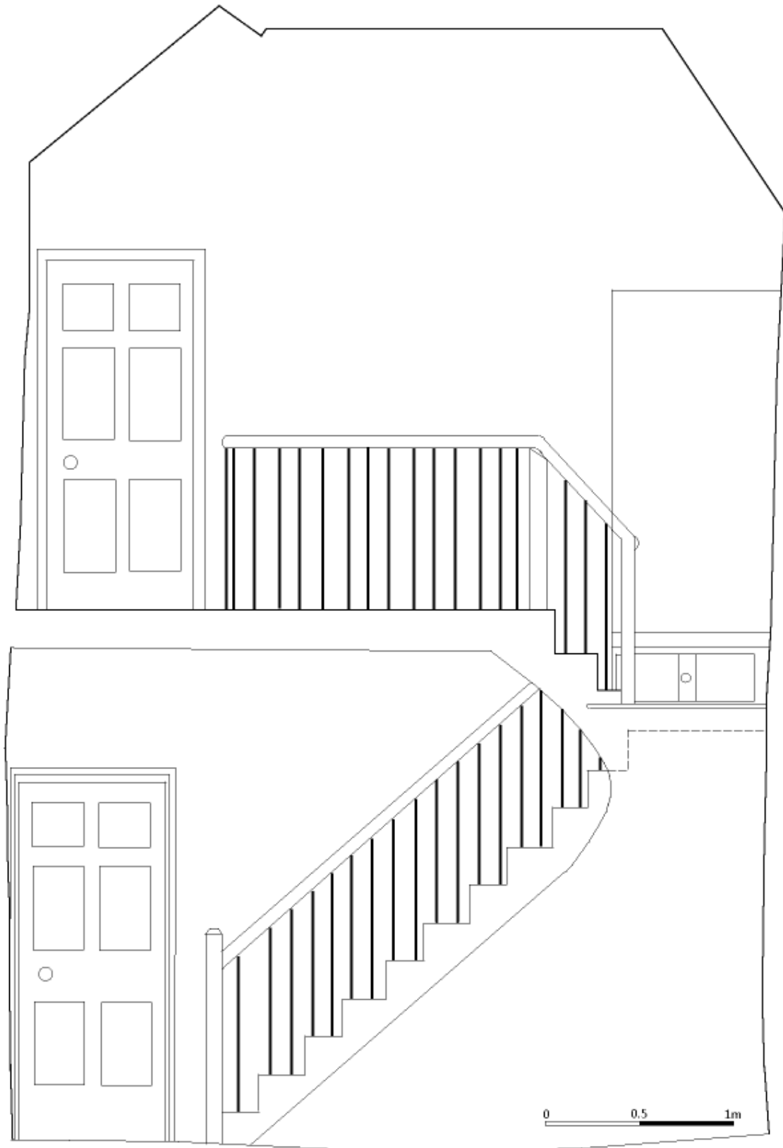
Fig. 7: Internal cross-section of first and second floors of main house looking NW showing dog-leg staircase and blocked doorway on half-landing
