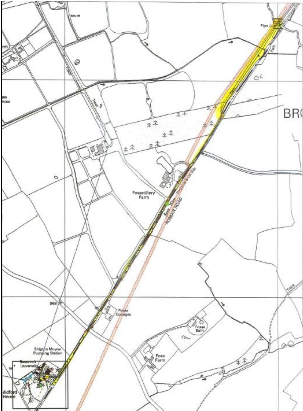
Fig 1: Plan showing the route of the proposed water mains pipeline running from the Shipton Moyne Pumping Station to the River Avon (marked in yellow) with an existing gas pipeline marked in red
