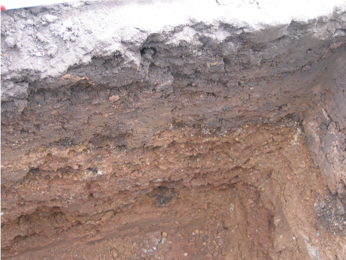
Plate 2: Section showing sand, gravel, clay and loam layers. Darker soil near surface may be tree-root disturbance.
