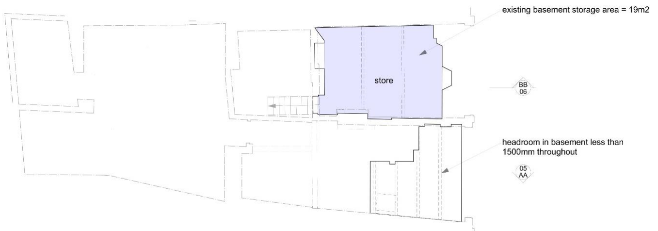
Fig 8: Plan of existing basement layout (Tillman Architects, dwg no. 230 01-01, Dec 2018)
