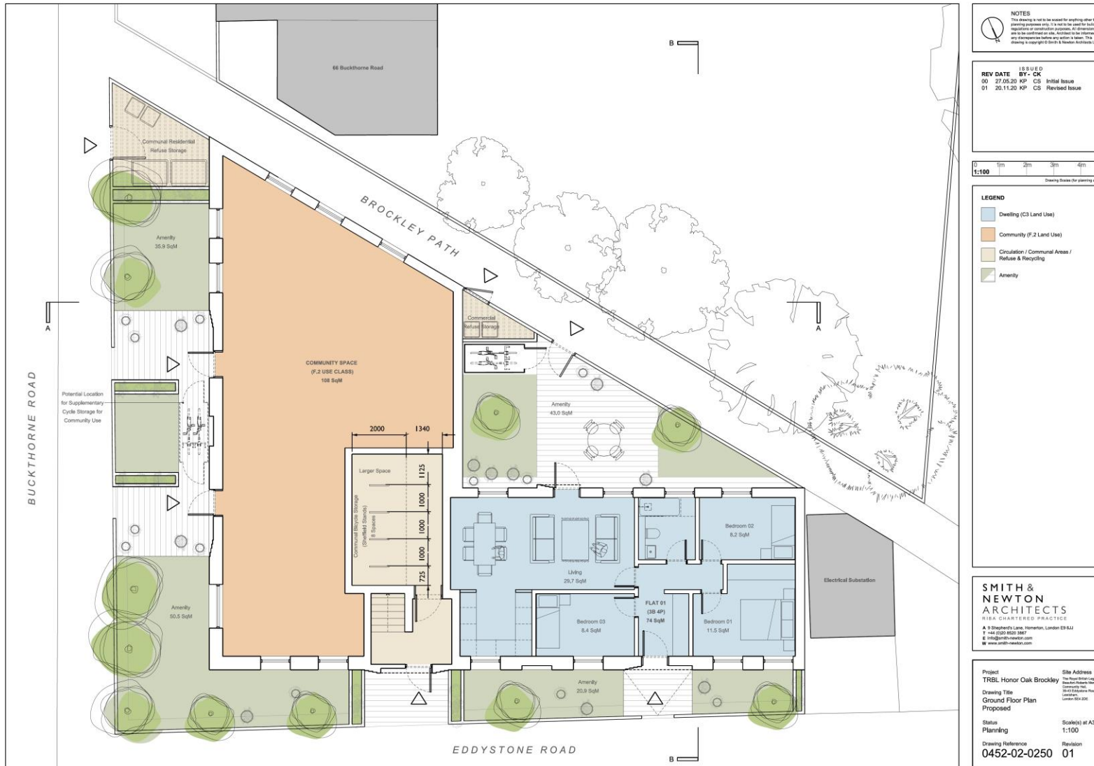
Fig. 5: Proposed ground floor plan of three storey mixed-use building at 39-43 Eddystone Road (Reproduced by courtesy of Smith and Newton Architects)
