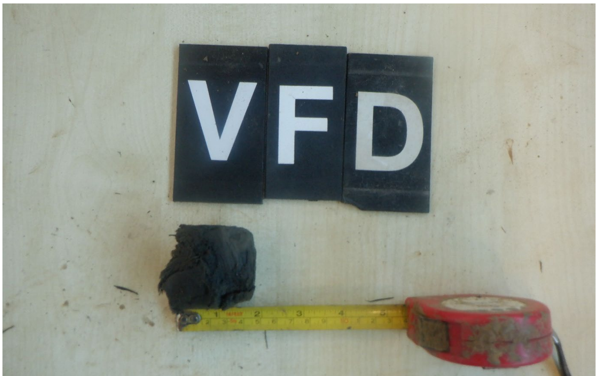
Plate 4: Additional parts of wood retrieved initially stuck within the barrel of the hand coring machine VC01.
