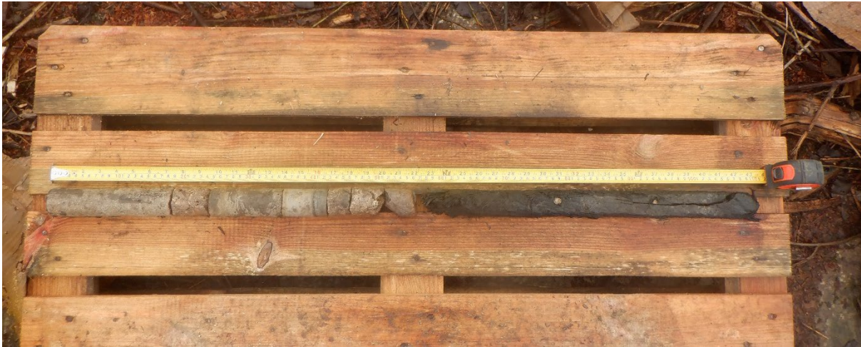
Plate 3: The sample retrieved from coring VC01 through the Scotland Weir. Note that the depth that the wood recovered from is unknown due to coring difficulties.
