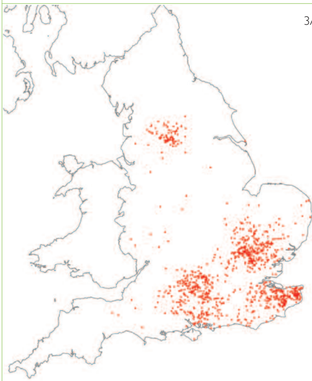
3 The distribution of listed aisled (left) and cruck (right) barns in England. Aisled construction, used for domestic buildings from the 12th century at the highest level in society, was suited to the storage and constructional requirements of large barns. The weighting of the distribution is southern English, stretching into the south of the East of England Region, with outliers being generally of a high status and dating from before 1550; a notable concentration in northern England is in the Halifax–Huddersfield area, where the wealth derived from a combination of farming and the cloth industry in the 15th and 16th centuries led to the construction of a notable group of aisled houses and barns. Aisled construction continued to be employed in southern England into the 19th century. Crucks in domestic buildings have a date range from the mid-13th to the mid-17th centuries, examples in the north of England being generally later in date, whereas in agricultural buildings the earliest survivals are 15th century and the latest (in the southern Pennines) early 18th century. There is a wide variety of forms in cruck construction. © Crown copyright. All rights reserved. English Heritage 100019088. 2005
