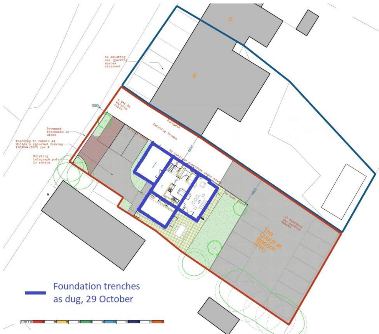
Figure 3: Detailed site location plan showing the positions of the foundation trenches dug on 29 October 2020. Measurements taken on site confirmed the accuracy of this plan, based on Colony Architects drawing 651 02-11. Scale 1:400 (original drawing 1:200).
