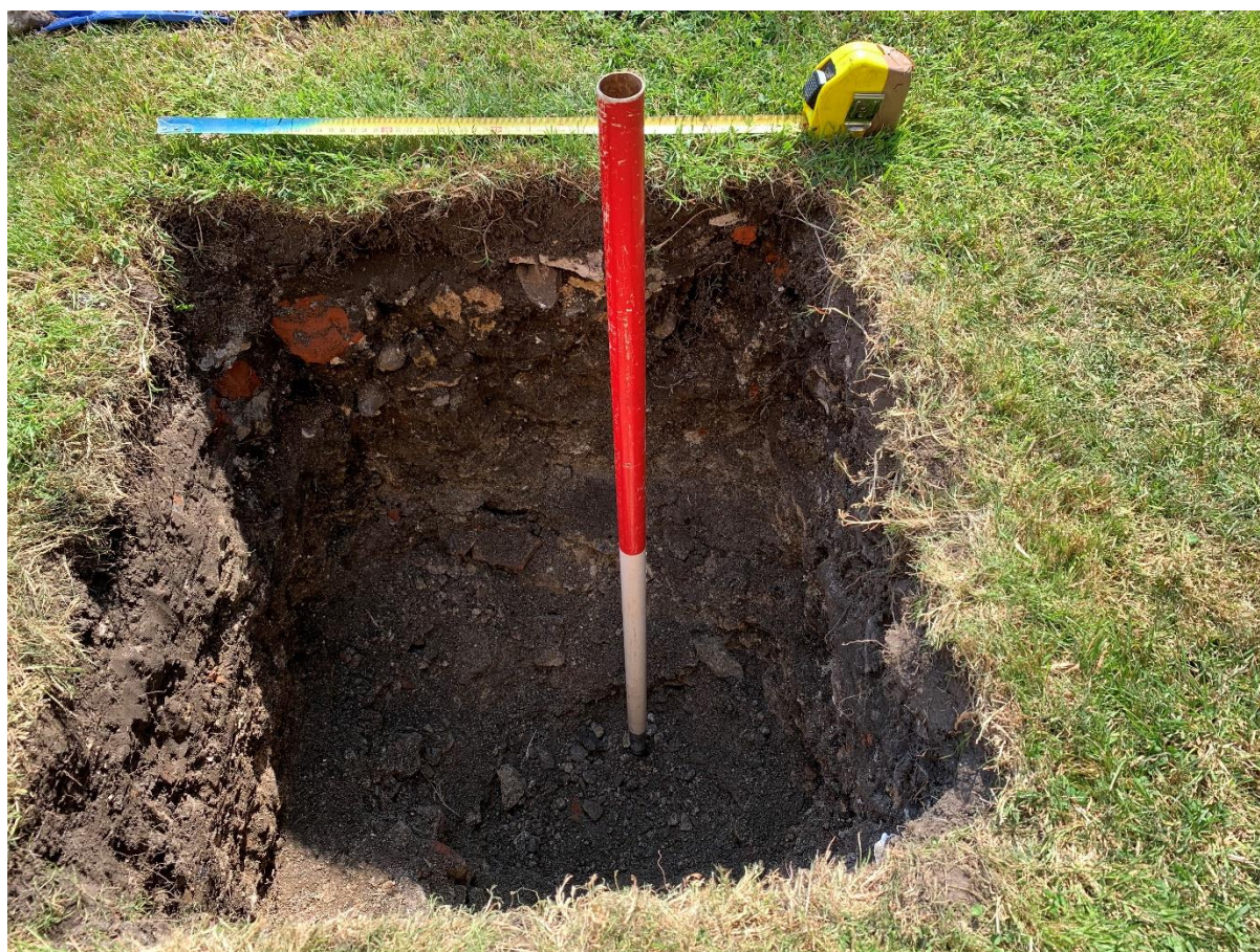
Figure 6: Pit 3 looking south, with rubble layer 10 occupying all but the top 80mm of the excavation.
