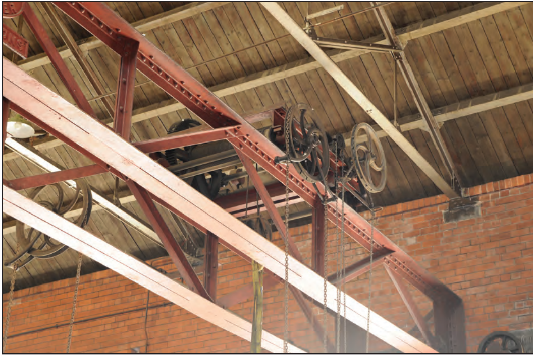
Photograph No. Washwood057 Description: Engine house travelling crane mechanism Site Location: C6c Direction From: below NW
