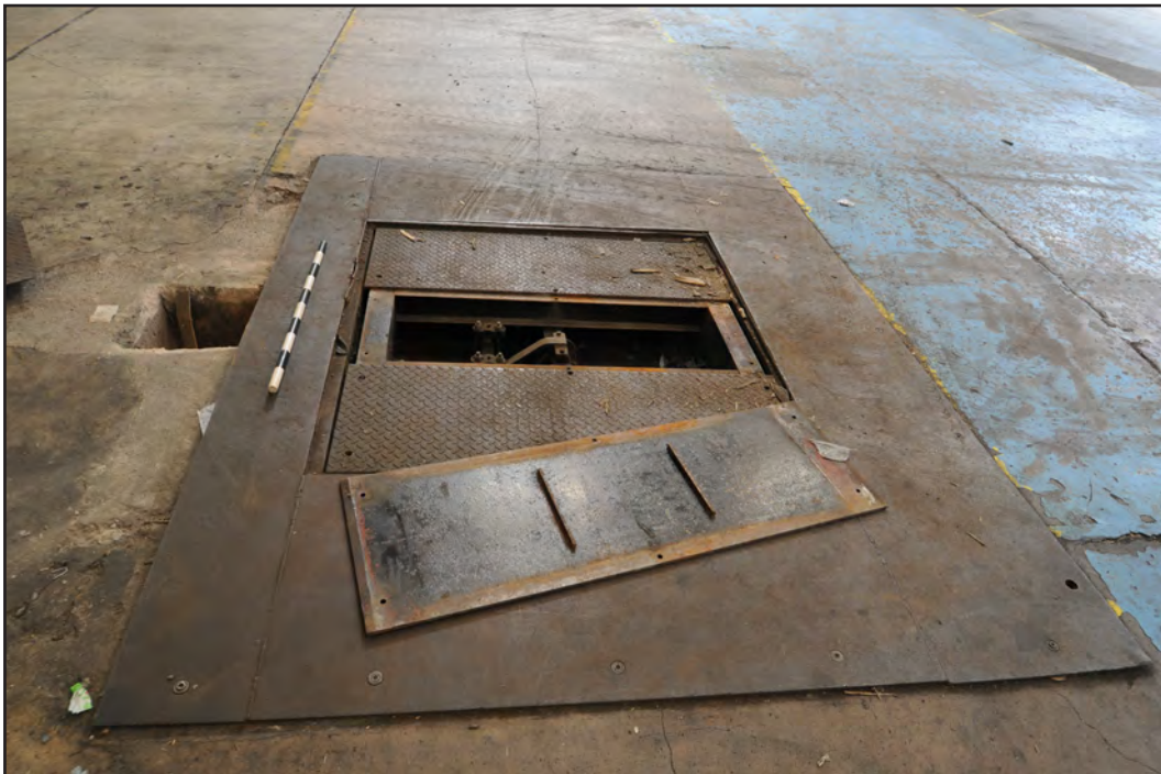
Photograph No. Saltley046 Description: Detail of weighbridge mechanism at northeast corner of interior Site Location: Anixter Direction From: N
