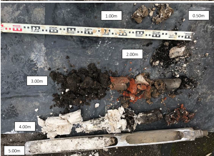
Plate 9: Borehole BH03 sample. (Photo from Advanced Investigations System Ltd 2020).
