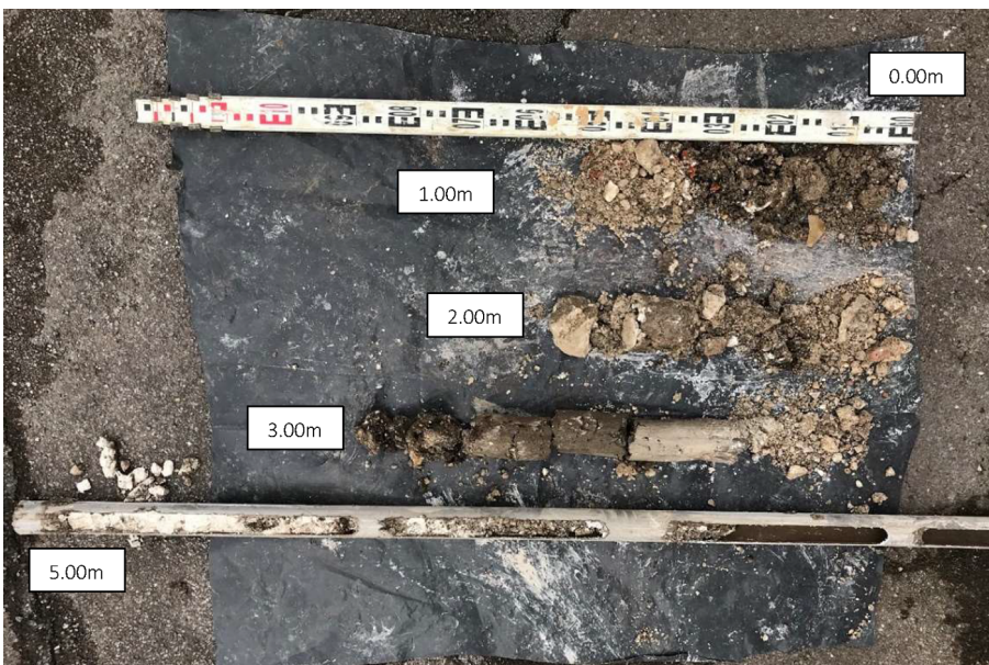
Plate 8: Borehole BH02 sample. (Photo from Advanced Investigations System Ltd 2020).
