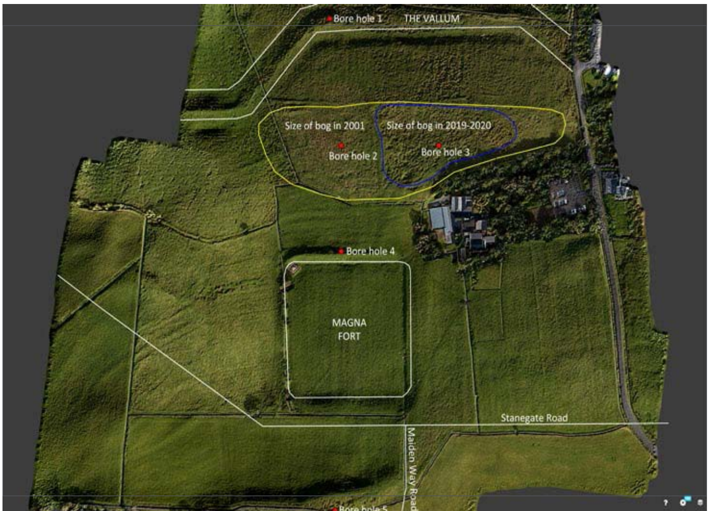
Figure 7: Proposed bore hole locations (red circles indicated the proposed bore hole locations). This composite image of Magna was taken in 2019 by SUMO archaeological services.
