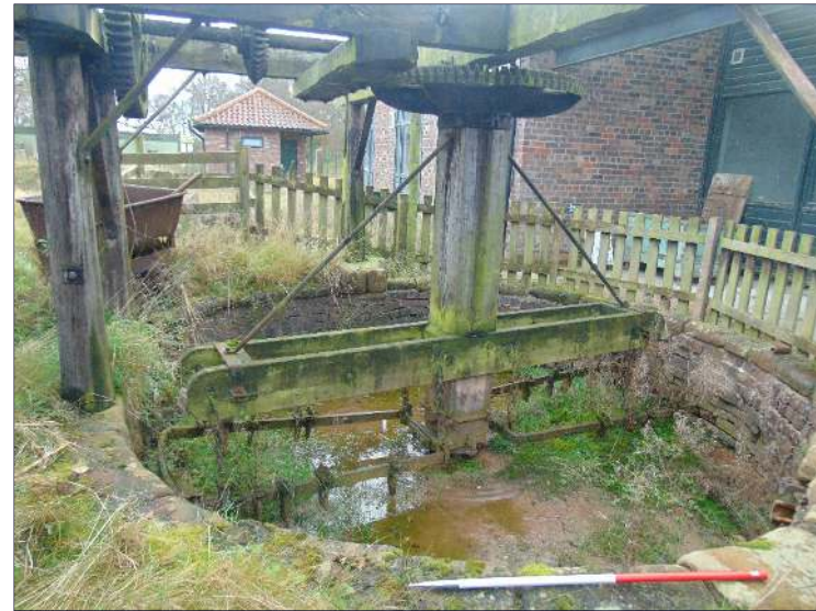
Plate 36: Blunger showing gearing and crown wheel, looking southeast [21]
