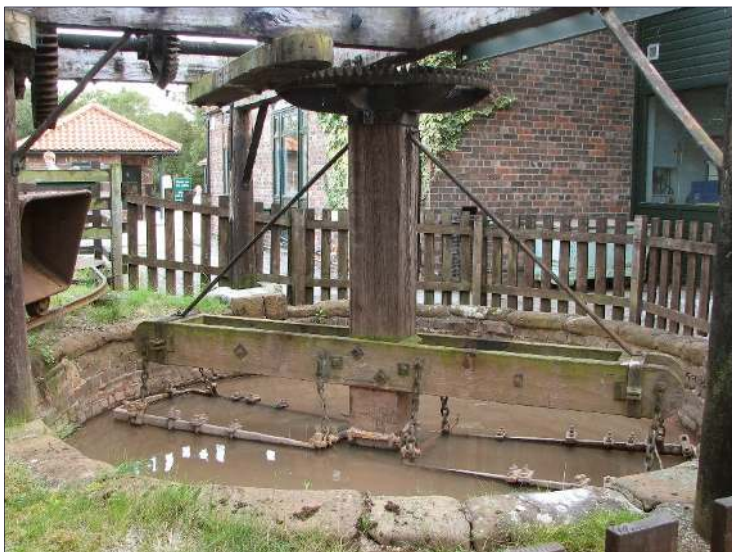
Plate 7: The blunger to the south of the engine house in 2007
