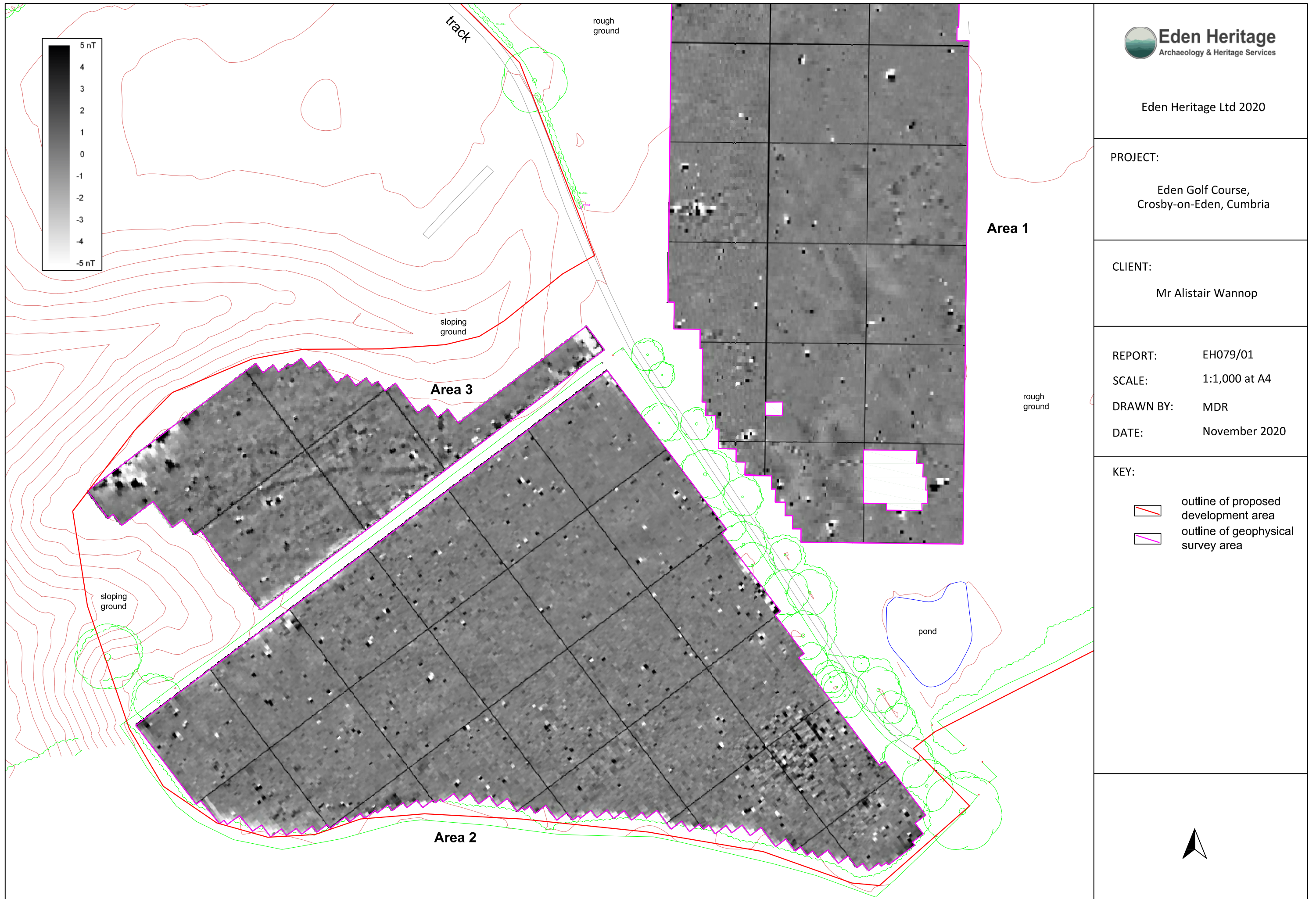
Figure 12: Geophysical survey of the south side of Area 1, Area 2 and Area 3 (minimally processed data) showing survey grid.
