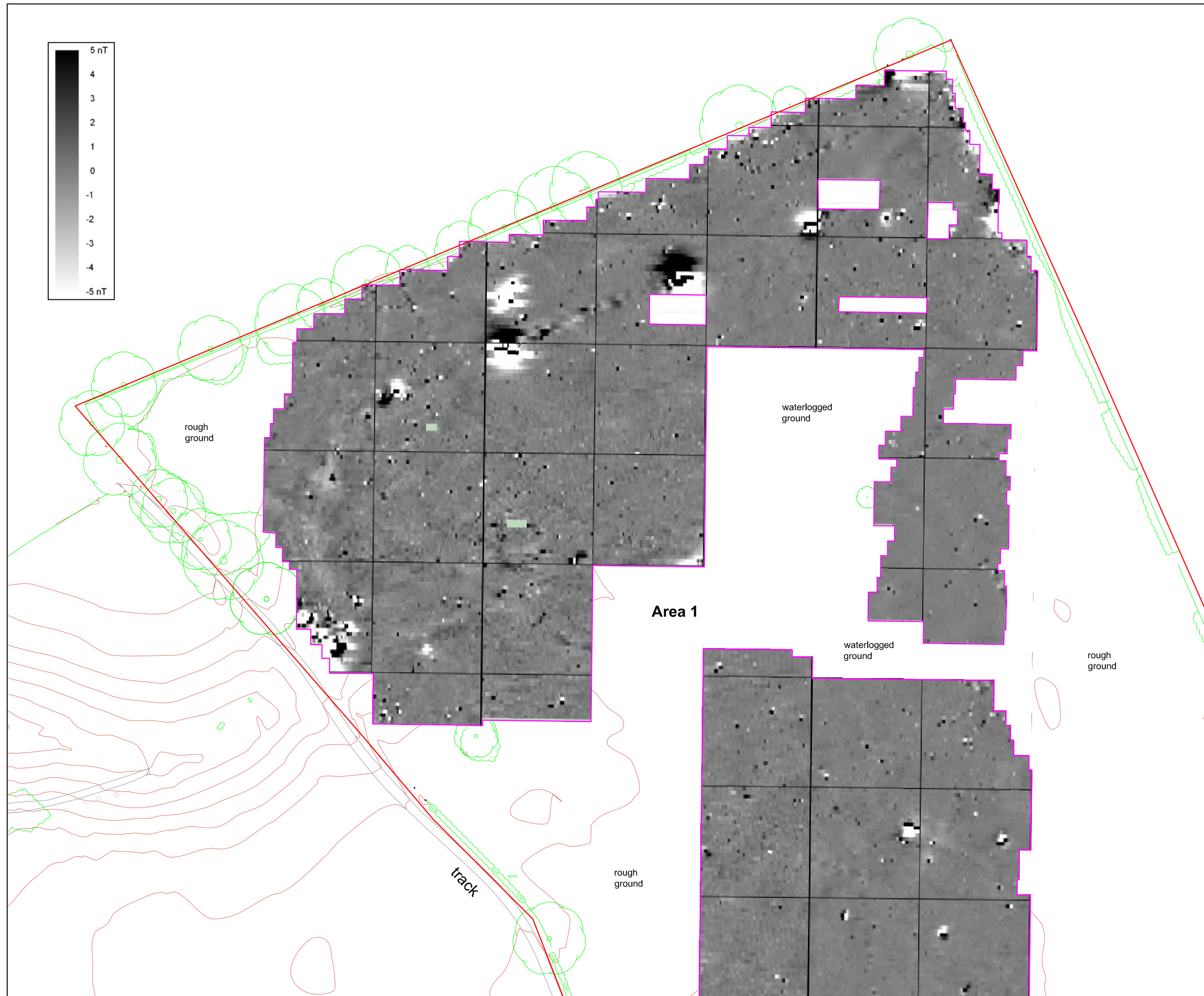
Figure 8: Geophysical survey of the north side of Area 1 (minimally processed data) showing survey grid.
