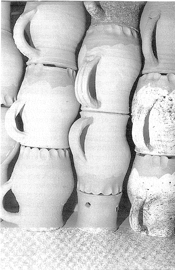
Pl. 1. Kiln stack. Non-overlapping uniform pots illustrating close packing by a contoured setting using a prop.
