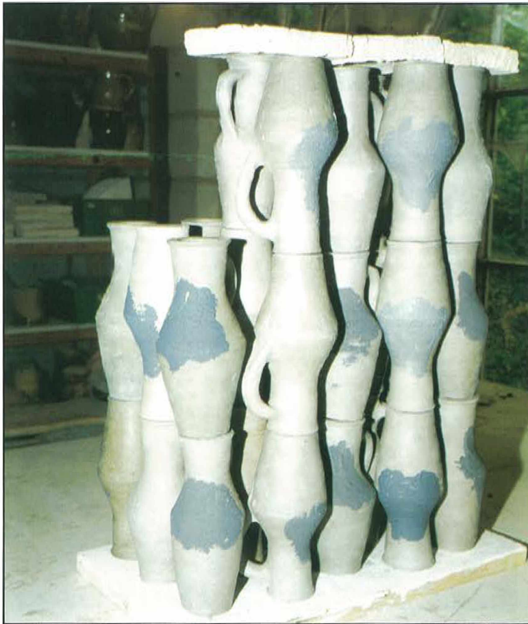
Colour Plate 5. a , Reduced cooking pots fired in the experimental kiln; b , mock-up of unfired Cheam-type drinking jugs showing close three-layer stacking and the position of the kiln capping on the topmost layer. A stack of four layers seems to be the maximum practical height. (See pp. 124–34).
