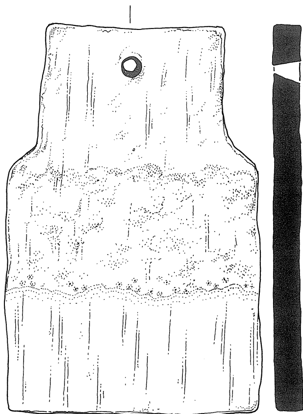
Fig. 1. Some roofing tile types used in medieval London: No. 1 shouldered tile. Scale: 1:4.
