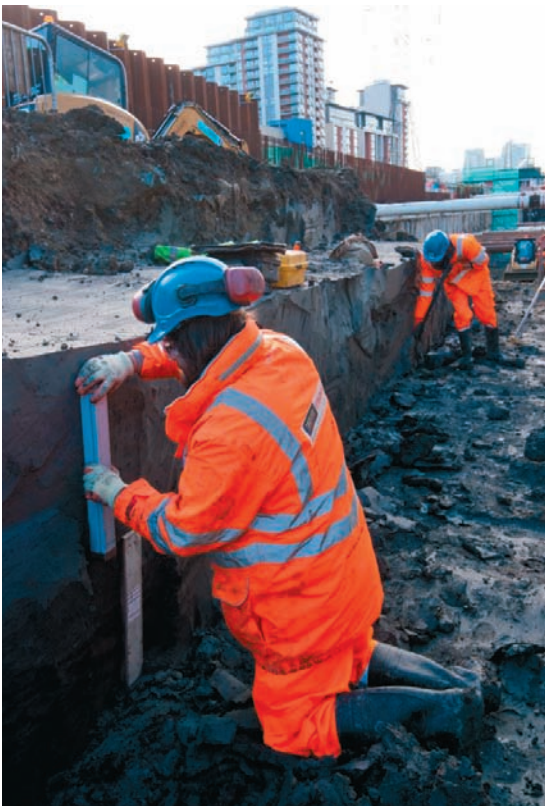
Fig 2 A geoarchaeologist sampling from a section through the organic complex and upper alluvial sequence at the North Woolwich Portal site, looking west
