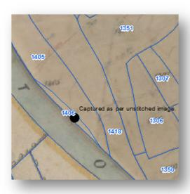
6. **Small polygon merged with plot.** A small, insignificant polygon has been included within an adjacent plot.
