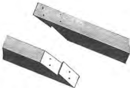
Fig. 9. Splayed and tabled scarf-joint (trait-de-Jupiter).
