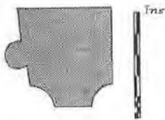
Fig 11. Profile of dais beam, reused as purlin in former Grammar School
